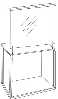
Step 5: Slide the pane into the grooves in the front mouldings. DO NOT glue. This panel allows access from the front.
